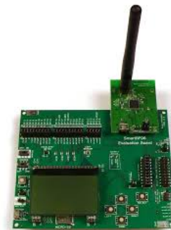
(b) Texas Instruments SmartRF06 EB and Texas Instruments CC2538 EM coupled.
