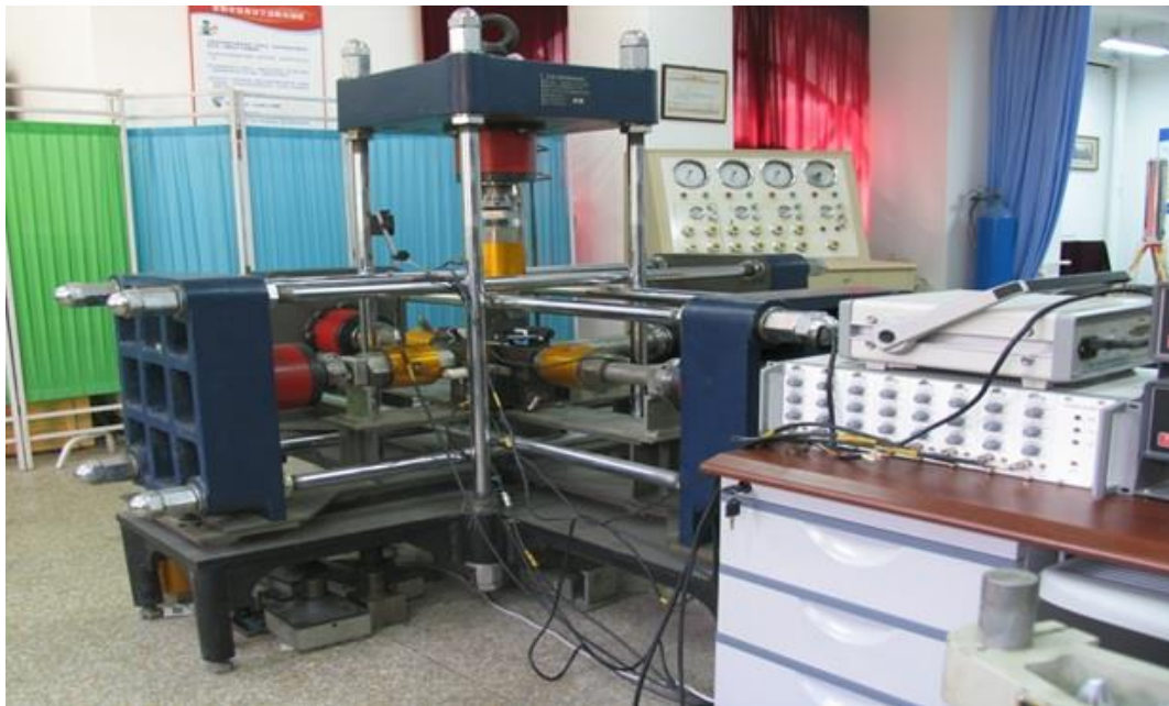
Figure 3: Rockburst laboratory testing system.
