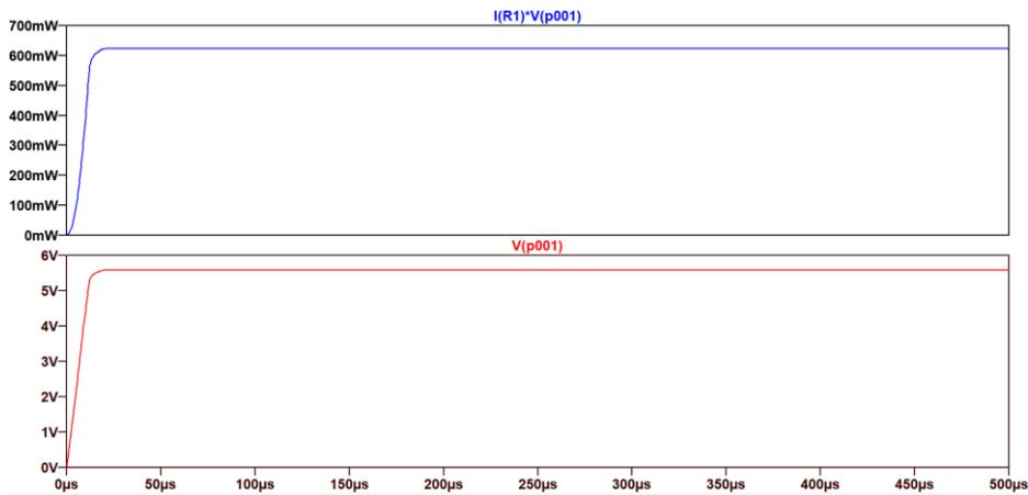
**Fig. 6.** Output power (624 mW) and voltage (5.58 V) in the equivalent circuit of the monocrystalline/polycrystalline module.
