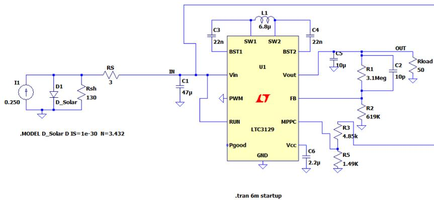
**Fig. 7.** LTC3129 converter between the model of the monocrystalline/polycrystalline module and the load.
