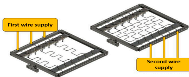
Figure 5. Drawer system with the positioning jig for the wires.
