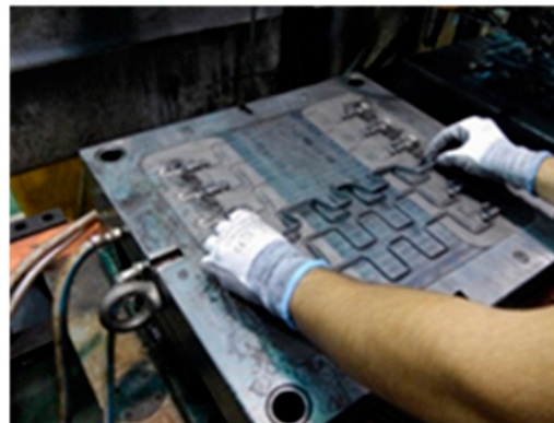
Figure 4. Operator inserting 2D bent wires into of the two lower half-mold. The over-molding is made on both tips of the bent wires (cavities).
