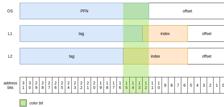
Figure 2.14: Disposition of colour bits in a 32-bits PA address from the point of view of an OS, L1 and L2 (PIPT) caches.
