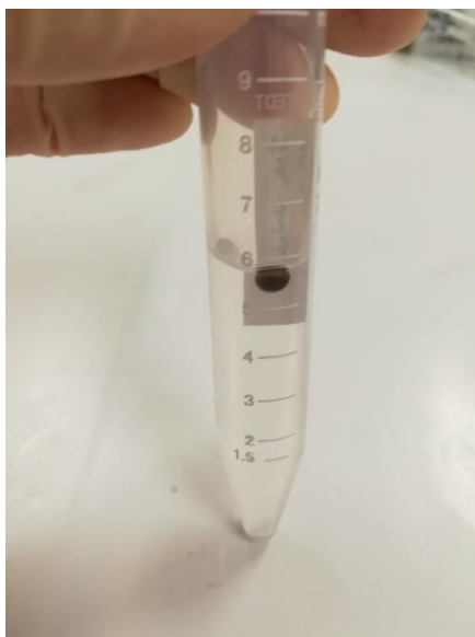
Figure 3.1. Preparation of solid magnetoliposomes. The water bubble contains the manganese ferrite nanoparticles cluster.
