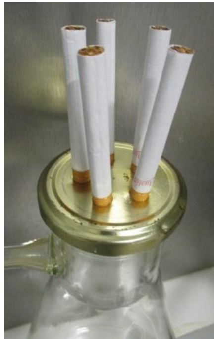
Figure 9. Cigarettes placed on the top of the Büchner flask.
