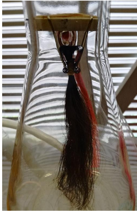
Figure 8. Support of the hair tresses on the Büchner flask.
