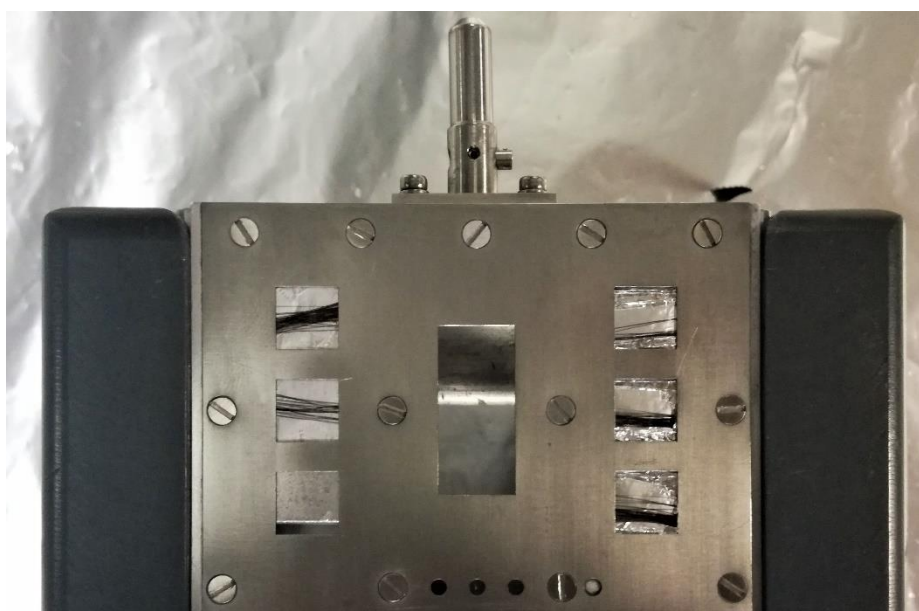
Figure 13. Samples assembling on the ToF-SIMS proper support.
