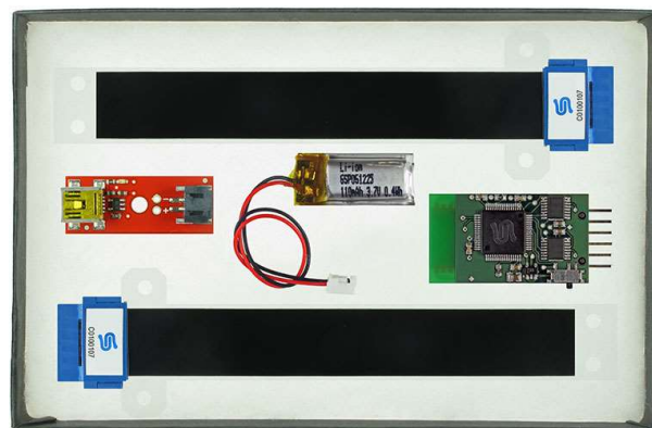
Figure 1 - : StretchSense „Evaluation-Kit, with the sensor bands (black stripes), the processing unit (right), battery (center) and USB adapter (left).
