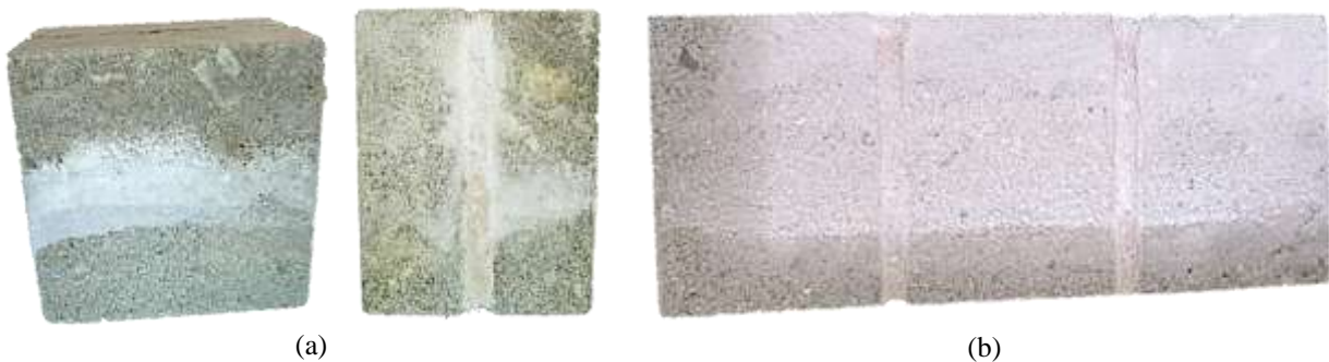
Figure 3. Visual aspect of masonry after the crystallization cycles on 10% NaCl water concentration; (a) duplet specimens; (b) triplet specimens
