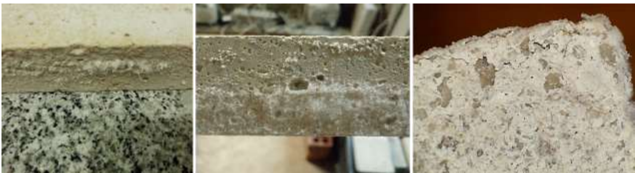
Figure 1. Lime mortar specimen subjected to 6 cycles in water with 10% NaCl concentration
