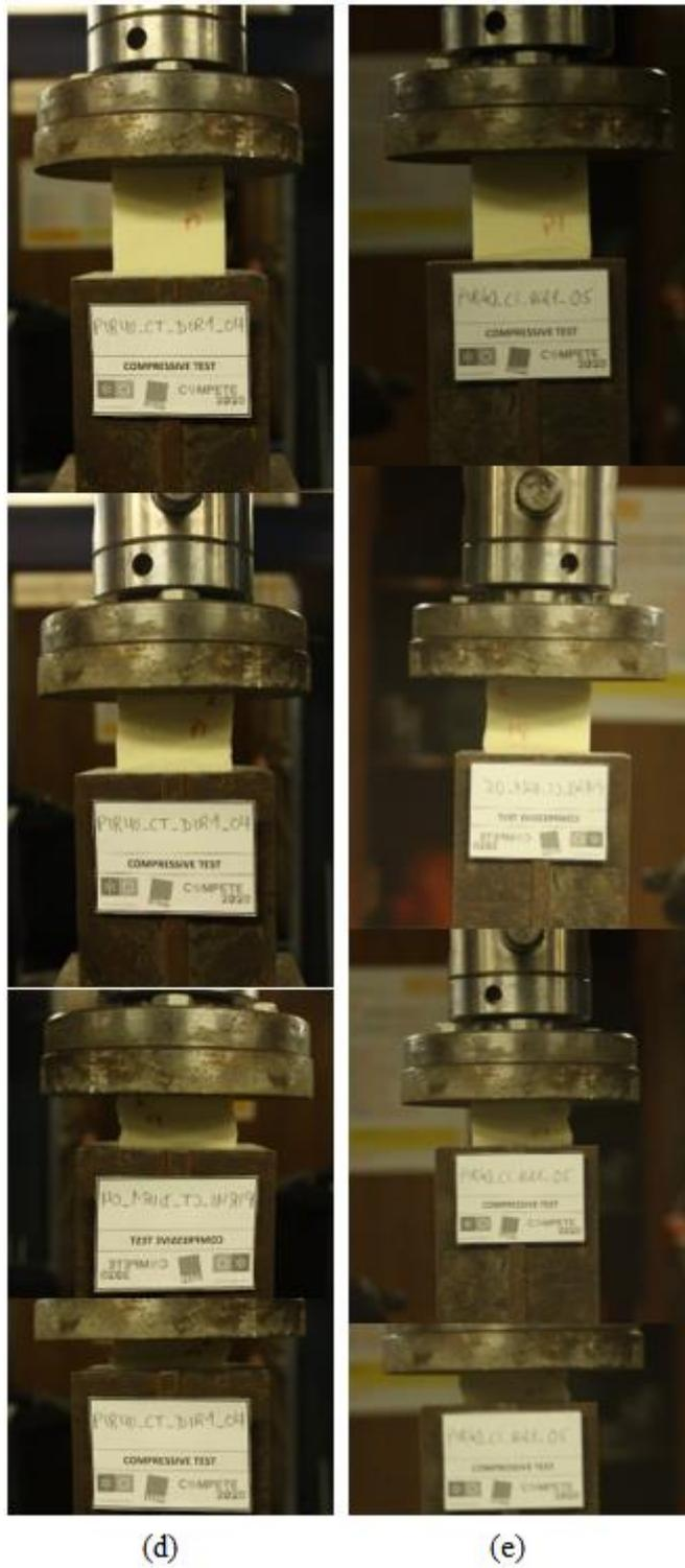
Figura V.2 – Modos de rotura: (a) PIR40\_CT\_01; (b) PIR40\_CT\_02; (c) PIR40\_CT\_03; (d) PIR40\_CT\_04; (e) PIR40\_CT\_05.
