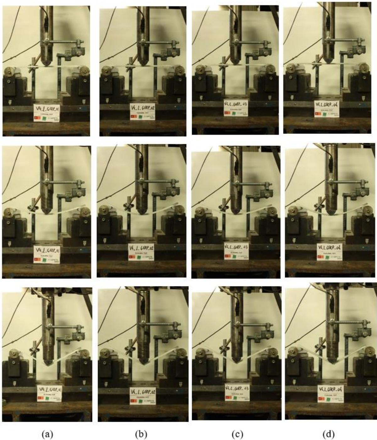
Figura II.1 – Modos de rotura: (a) V1\_GFRP\_L\_01; (b) V1\_GFRP\_L\_02; (c) V1\_GFRP\_L\_03; (d) V1\_GFRP\_L\_04.
