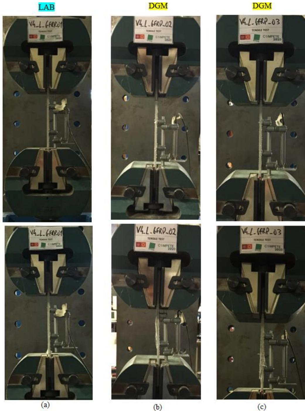
Figura III.1 – Modos de rotura: (a) V1\_GFRP\_L\_01; (b) V1\_GFRP\_L\_02; (c) V1\_GFRP\_L\_03.
