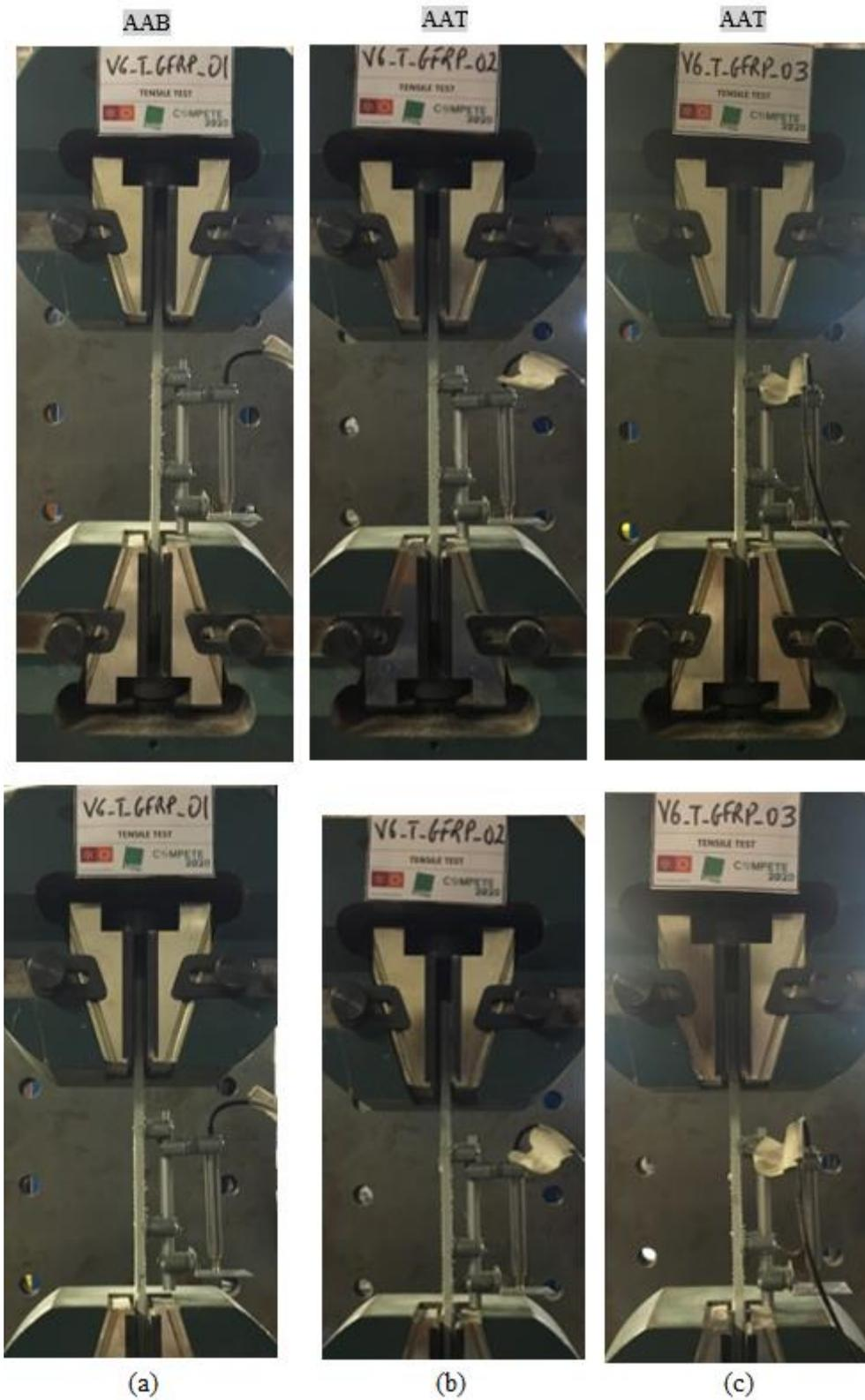
Figura III.6 – Modos de rotura: (a) V3\_GFRP\_T\_01; (b) V3\_GFRP\_T\_02; (c) V3\_GFRP\_T\_03.
