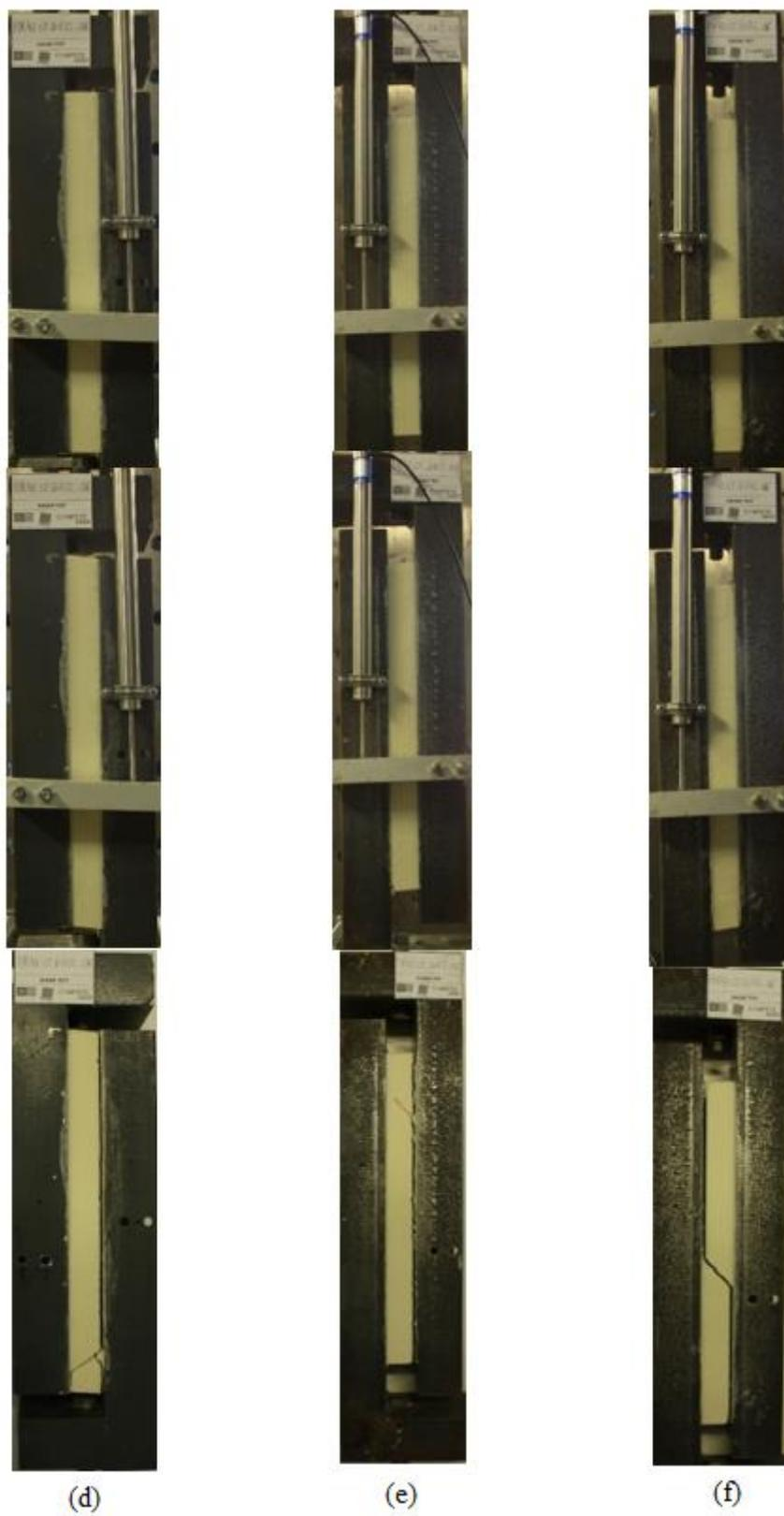
Figura VI.2 – Modos de rotura: (a) PIR40\_ST\_01; (b) PIR40\_ST\_02; (c) PIR40\_ST\_03; (d) PIR40\_ST\_04; (e) PIR40\_ST\_05; (f) PIR40\_ST\_06.
