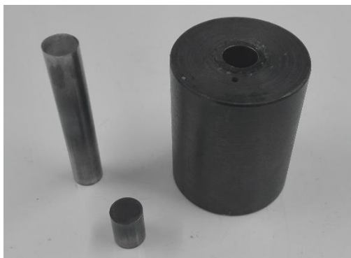
Figure 33 – Steel mold and punches used to process the materials
