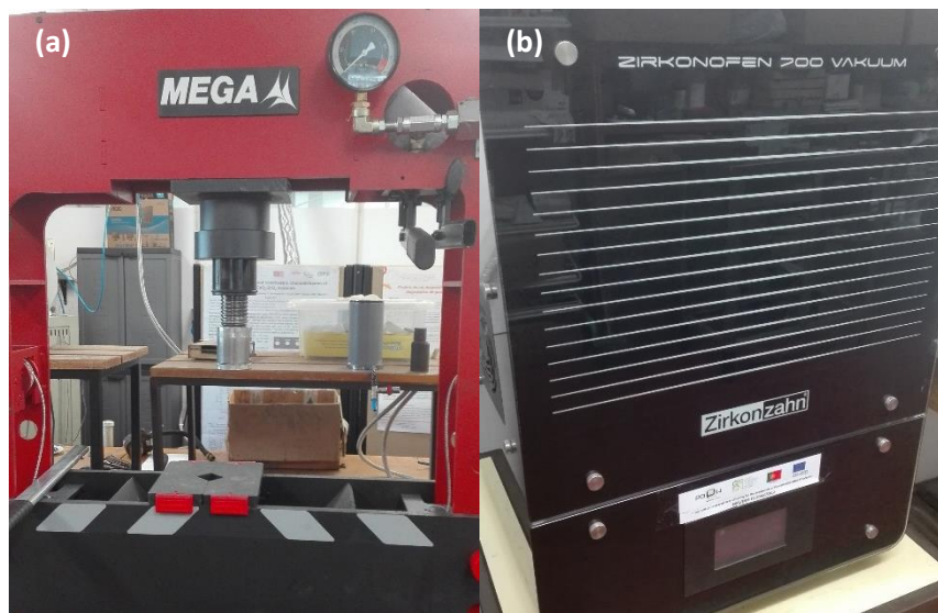
Figure 34- (a) hydraulic press (Bb) Zirkonofen 700 ultra-vacuum sintering furnace.
