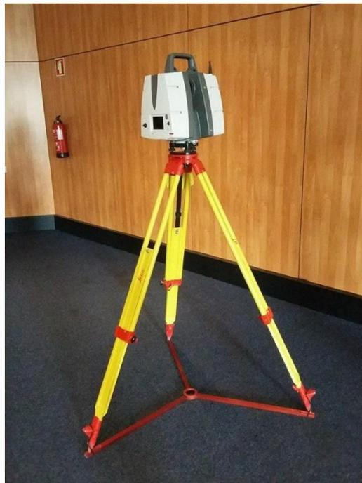
Figura 18. *Laser Scanning* – Leica P40.
