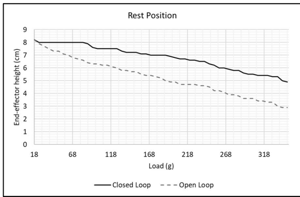
Fig. 9. End-effector positions, in function of the initial one, versus the load manipulated at the manipulator rest position.
