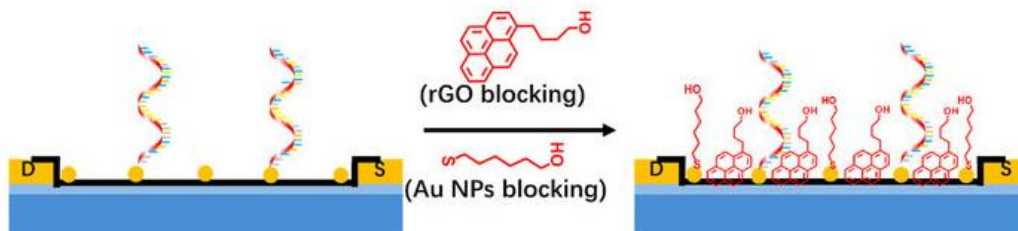
Figure 53: Schematic representation of a redox reaction detection on a functionalized FET gate, which the released electron activates a flowing current through the device. The amount of produced current is proportional to the binding reaction between the aptamer and the biomarker (Xiaoyan Chen et al., 2019).
