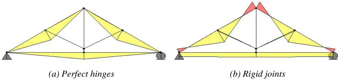
*Fig 3 Bending moment diagrams for self-weight load case*
