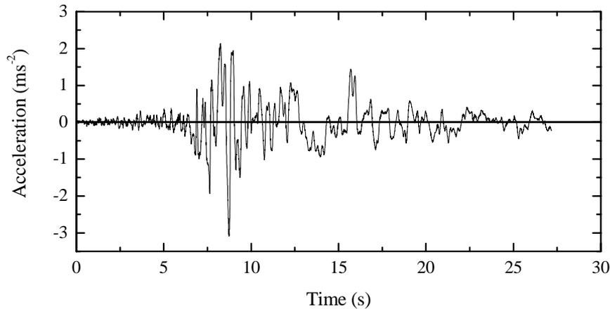
Fig 10 Accelerogram corresponding to the Kocaeli earthquake, Turkey (1999), Duzce station
