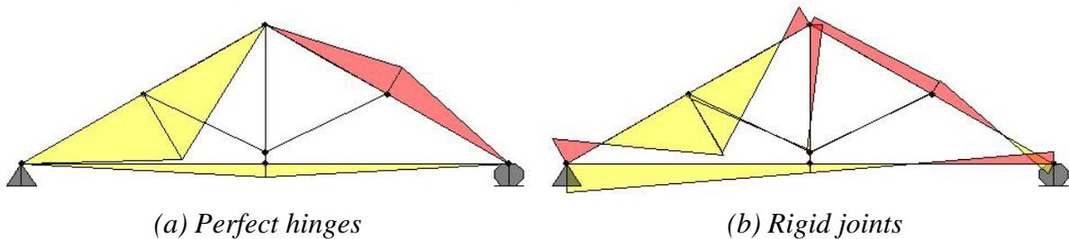
*Fig 4 Bending moment diagrams for snow load case*
