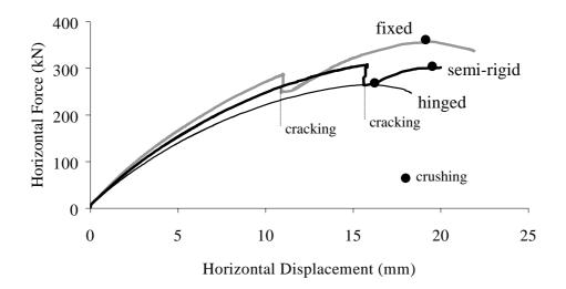
Fig. 5 – Typical results of the numerical simulation for different connection stiffness (l/h =
