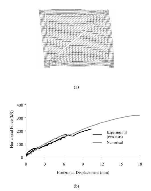
Fig. 3 – Typical results of the numerical simulation (panel with h / l = 0.83): (a) deformed mesh with separation between frame and panel, and with cracked panel;
