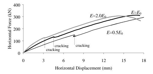
Fig. 7 – Typical results of the numerical simulation for different masonry stiffness (l/h = 1.00)
