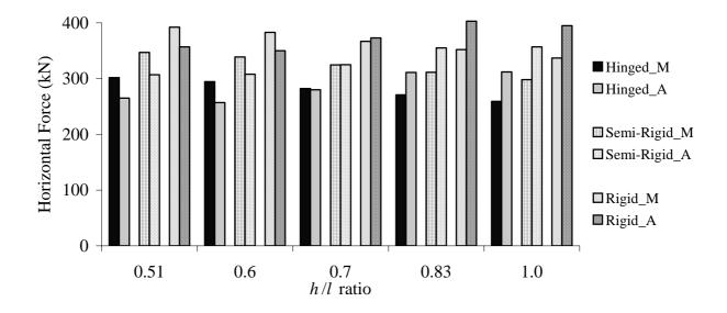
Fig. 12 – Comparative analysis between the results obtained for the force leading to crushing of the compressed corner, in the case of different h / l ratios and different connection stiffness
