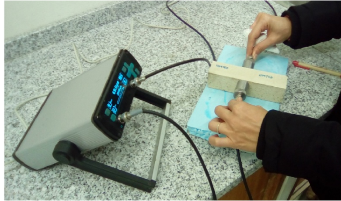
225 Figure 5: UPV set-up. Discrete measurement in the lateral direction.
