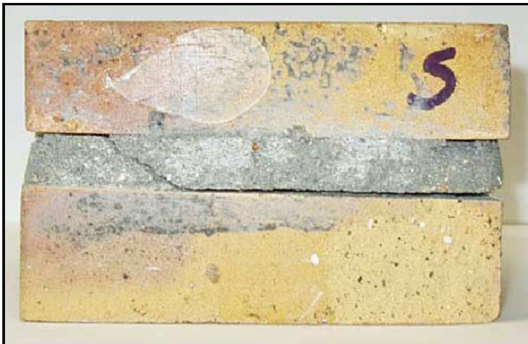
Figure 18 Failure mode during shear test (Abdou et al., 2006)
