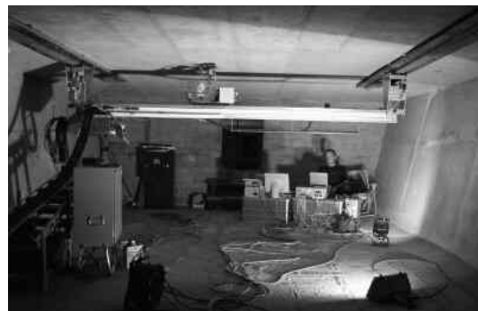
Figure 3.8 - Scanner system under development for automated measurements of radar, ultrasonic and impact-echo in parallel traces (x- and y-direction) at BAM ( www.bam.de )
