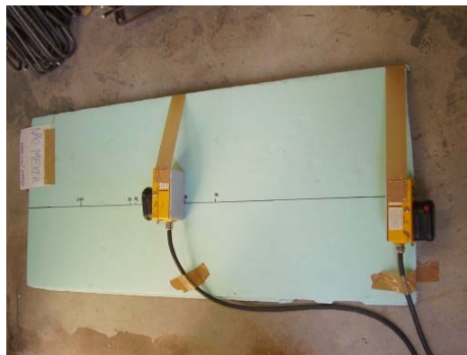
Figure 4.19 - Configuration of the MALA antennas for the air measurement
