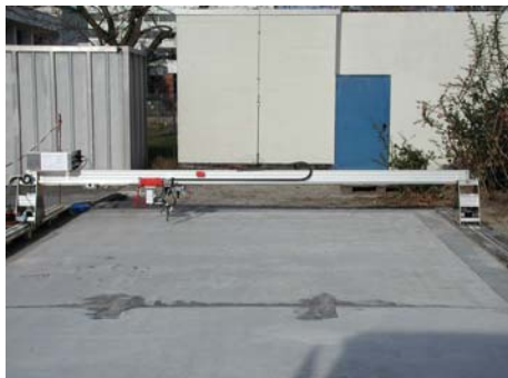
Figure 3.8 - Scanner system under development for automated measurements of radar, ultrasonic and impact-echo in parallel traces (x- and y-direction) at BAM ( www.bam.de )
