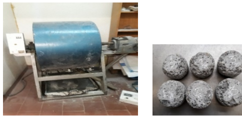
Fig. 8. Los Angeles machine and result of the test of Cantabrian
