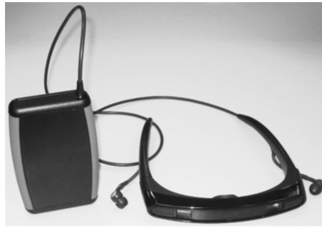
Figure 9.: Virtual (augmented) reality goggles used in ( Espay et al, 2010 (4) ) containing built-in LCD screen which projects floor tiles when subjects are moving, and earphones that sound step-matched cues as determined by connected sensor strapped as belt
