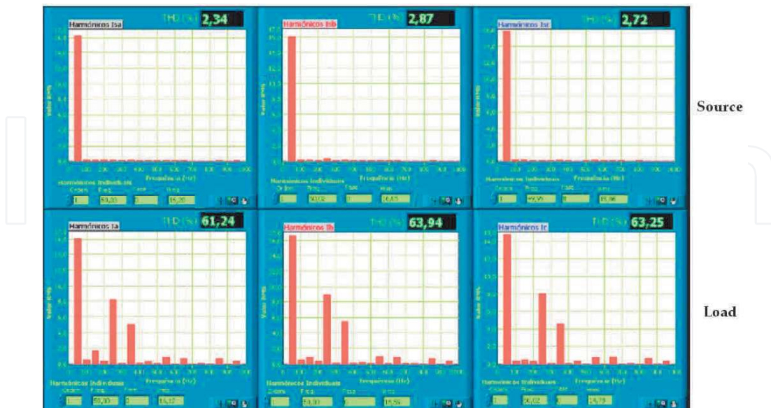
Figure 19. Current harmonics and THD% at Load and Source sides of the Shunt Active Power Filter, registered in installation 1 (Textile Industry).
