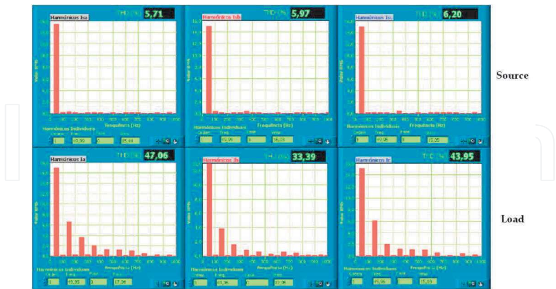
Figure 21. Current harmonics and THD% at Load and Source sides of the Shunt Active Power Filter, registered in installation 2 (Computational Center).
