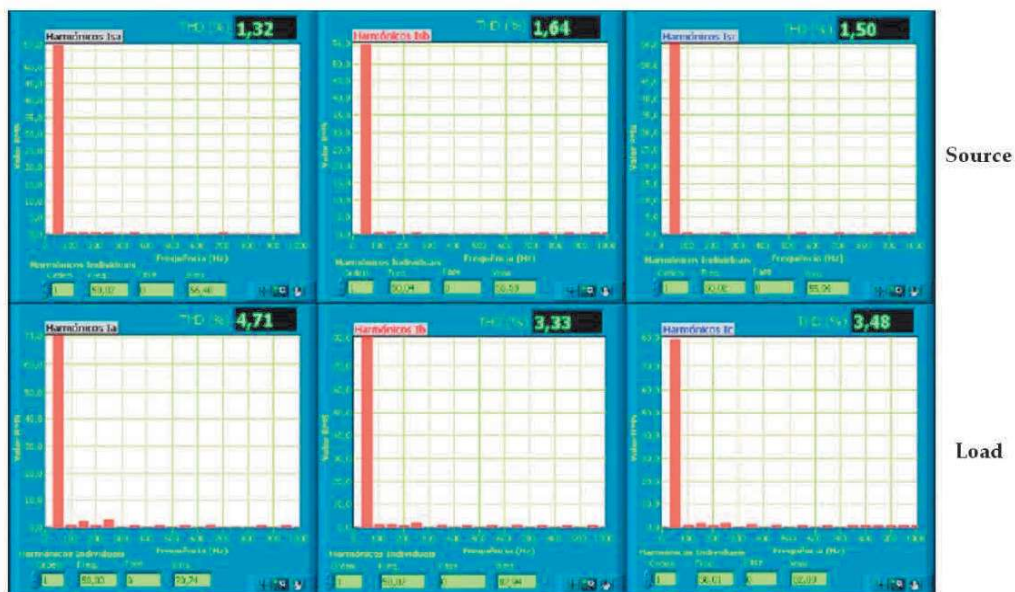
Figure 25. Current harmonics and THD% at Load and Source sides of the Shunt Active Power Filter, registered in installation 4 (Medical Drugs Distribution Warehouse).
