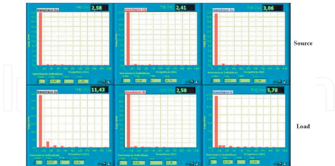
Figure 23. Current harmonics and THD% at Load and Source sides of the Shunt Active Power Filter, registered in installation 3 (Clinical Analysis Laboratory).
