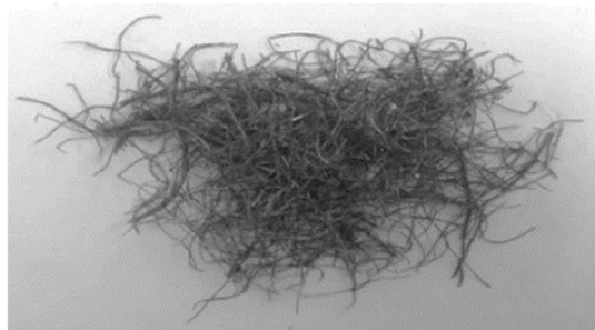
Figure 2.6 - RSF obtained from cryogenic process (Zamanzadeh et al. , 2015)
