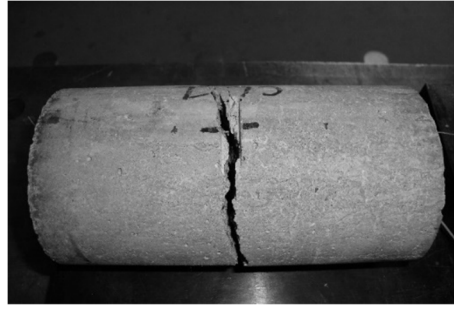
Figure 5.7 – Specimen of Series IV after four-point load bending test
