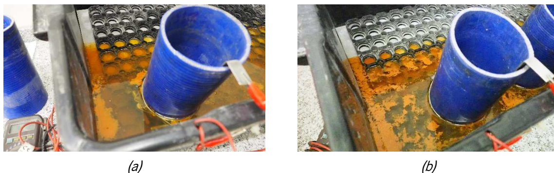
Figure 7.45 – Chloride migration tests carried out with specimens made with: (a) The RSFRC1%_2 casting and (b) The RSFRC1%_4 casting
