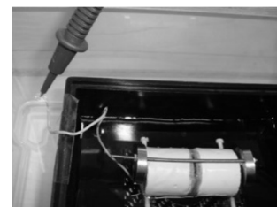
Figure 5.14 – (a) (b) Chloride immersion of cracked mortar specimen under tension; (c) Electrochemical monitoring of embedded RSF into mortar specimen
