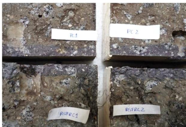
Figure 7.47 – Chloride penetration depth in RSFRC and PC cubes after 3 months of immersion
