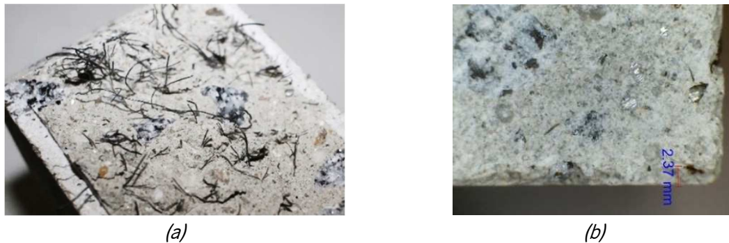
Figure 6.19 – Crack surface of specimens after 6 months of chloride immersion (Series VI): (a) General aspect of RSF; (b) Corrosion sign on RSF near the exposed surface
