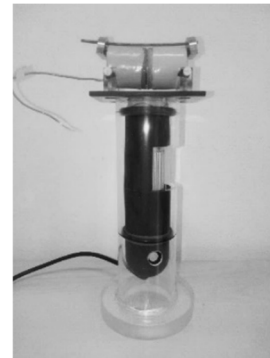
Figure 5.13 – (a) Supporting and load application systems for cracked mortar specimens; (b) Measurement of crack width with a microscope (units in mm)
