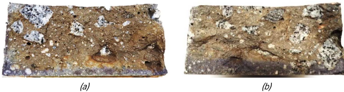
Figure 7.9 – Split section of PC cylindrical specimens: (a) after 10 days of immersion (b) after 3 months of immersion
