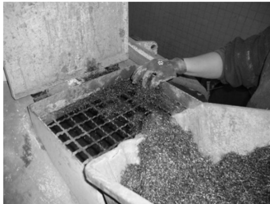
Figure 3.24 – Introduction of RSF into the concrete mixer
