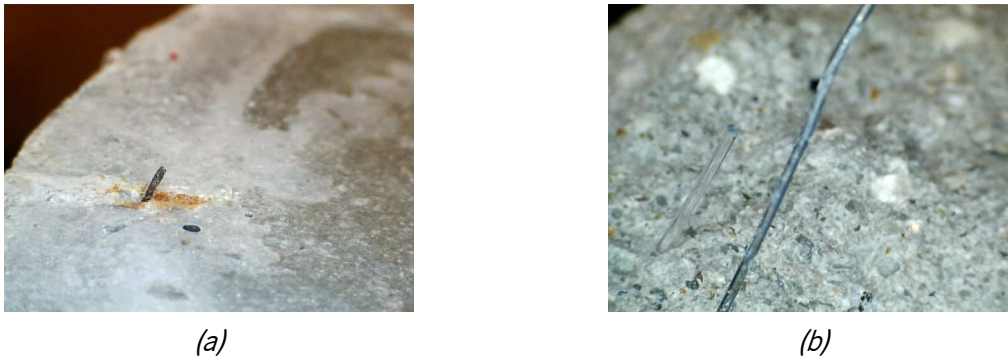
Figure 5.9 – Aspect of RSF after fiber pull-out test of: (a) SP1 (Series I); (b) SP11 (Series IV)
