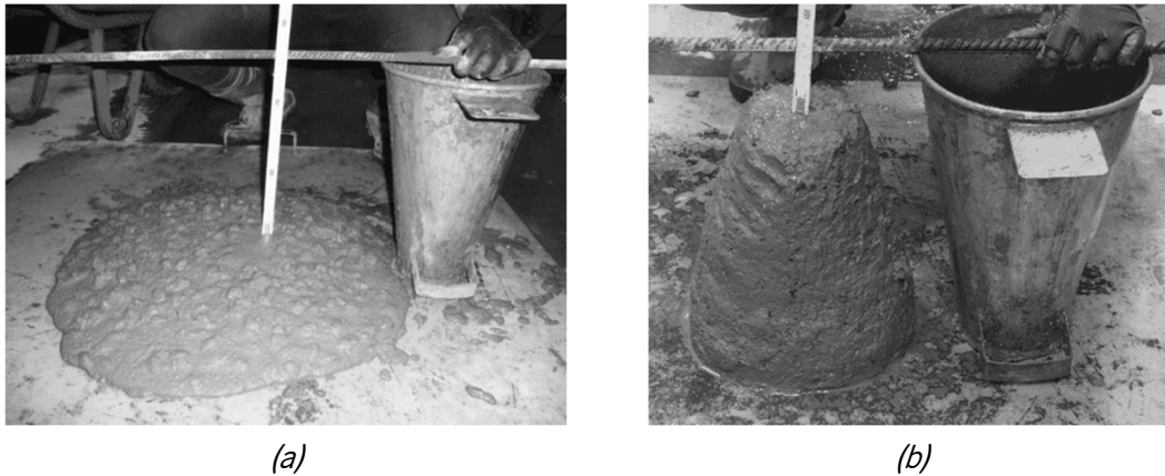
Figure 3.25 – Slump tests for a concrete reinforced with 76 \text{ kg/m}^3 of RSF (a) Before and (b) After the addition of the RSF
