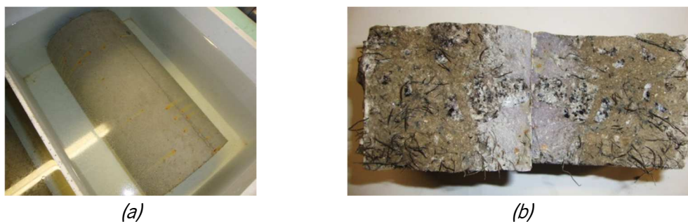
Figure 6.14 – Specimens after 3 months of chloride immersion (Series V): (a) Aspect of 3.5% NaCl solution and corrosion spots at exposed faces (b) Chloride penetration depth
