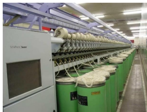
Figura 13 - Continuo de anel open-end (Barbosa, 2012) .
