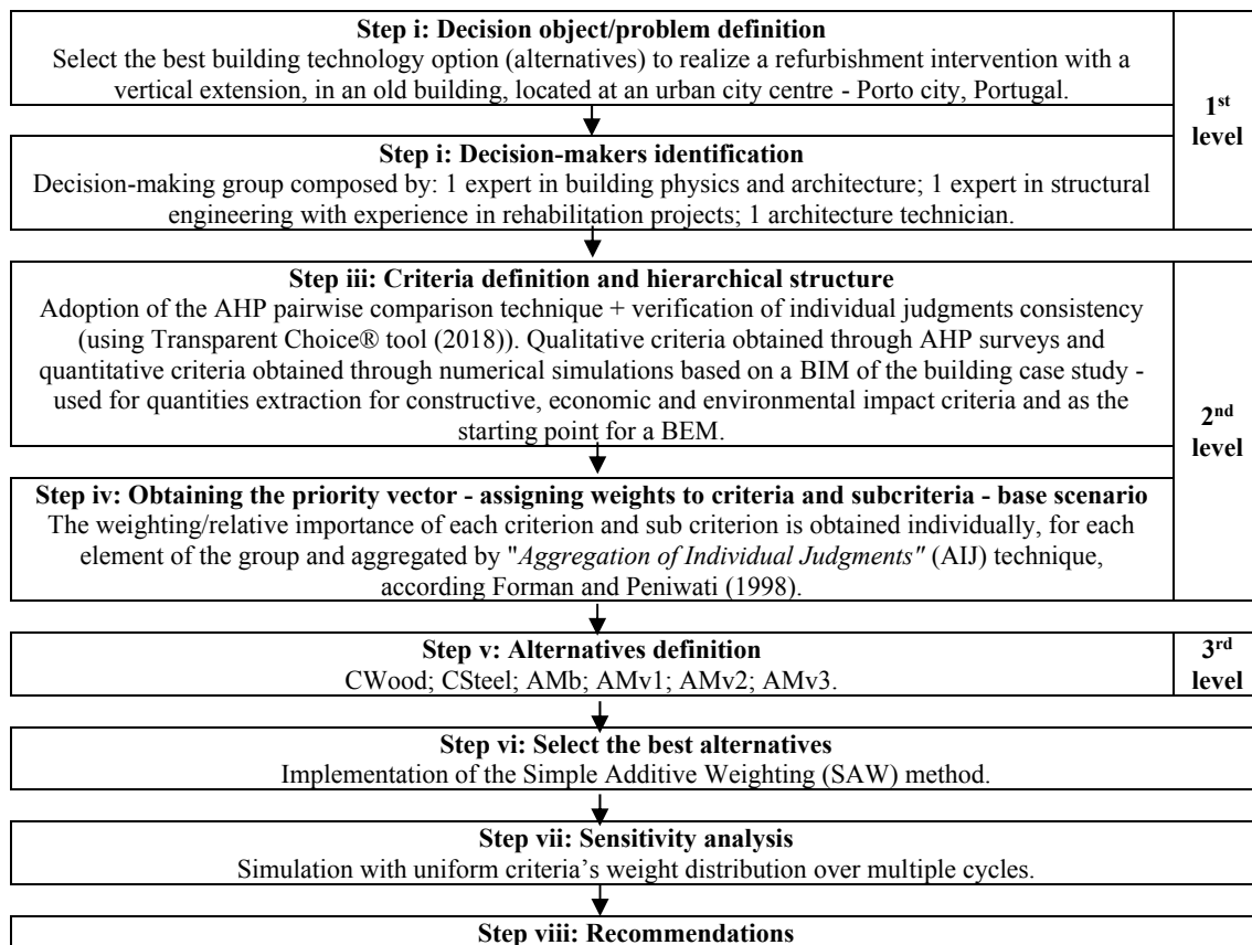
Figure 3. Flowchart of the adopted decision analysis process in the present case study (adapted from Clemen and Reilly (2001)).
