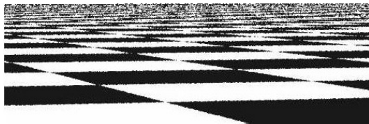
(a) Jittered sampling with 1 sample per pixel.
