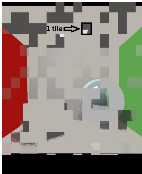
Figure 16.: Illustration of tiling the image plane.
