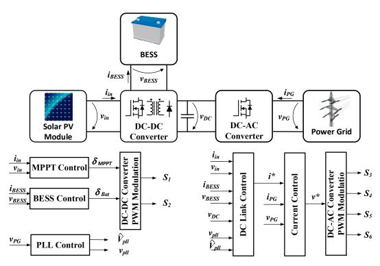
Figure 7. Block diagram of the microinverter with the integration of the control algorithms.
