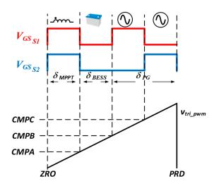
**Figure 2.** Signal sequence to obtain the pulse-width modulation (PWM) signals for the semiconductors  $S_1$  and  $S_2$ .
