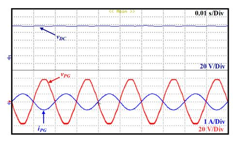
**Figure 19.** Experimental results of the developed multifunctional isolated microinverter: oltage at the DC-link ( $v_{DC}$ ), voltage ( $v_{PG}$ ) and current ( $i_{PG}$ ) on the power grid.
