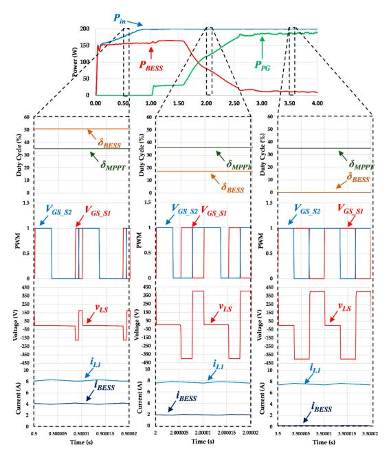
**Figure 10.** Identifiable influence of the  $\delta_{MPPT}$  and  $\delta_{BESS}$  control variables from the MPPT and BESS charging control algorithms at different time intervals:  $V_{GS\_S1}$ —MOSFET  $S_1$  gate–source PWM signal;  $V_{GS\_S2}$ —MOSFET  $S_2$  gate–source PWM signal;  $v_{LS}$ —voltage at the secondary winding terminals of the high-frequency transformer;  $i_{L1}$ —input current measured on inductor  $L_1$ ;  $I_{BESS}$ —BESS charging current.
