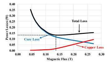
Figure 14. Power losses of the high-frequency power transformer.
