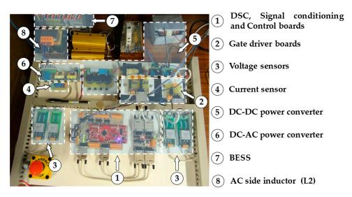
Figure 12. Top view of the developed multifunctional isolated microinverter prototype.
