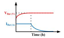
**Figure 5.** Representation of the two stages of the constant current followed by the constant voltage control algorithm.
