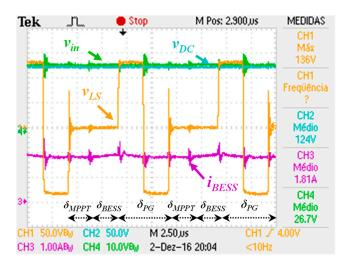
**Figure 17.** Experimental results of the DC–DC power converter:  $v_{DC}$ ,  $v_{in}$ ,  $v_{LS}$  and  $i_{L1}$  with the MPPT and the BESS control algorithms enabled.
