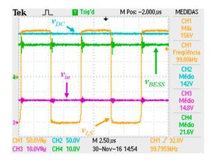
**Figure 15.** Experimental results of the DC–DC power converter: Input voltage ( $v_{in}$ ), BESS voltage ( $v_{BESS}$ ), DC-link voltage ( $v_{DC}$ ) and secondary winding voltage ( $v_{LS}$ ) when the transformer operates with a 50% duty cycle.
