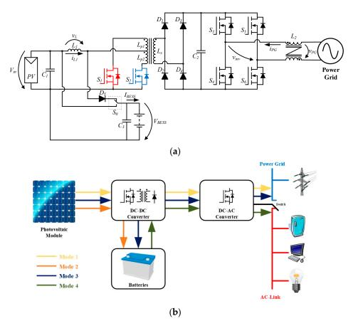
**Figure 1.** Topology and operation modes of the proposed multifunctional isolated microinverter: (a) Schematic of the microinverter topology; (b) Representation of the operation modes.
