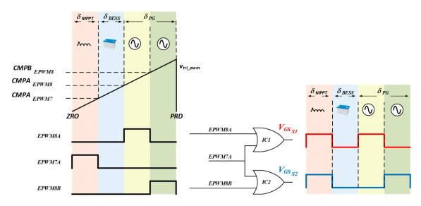
**Figure 13.** Circuit used to obtain the PWM signals for the semiconductors  $S_1$  and  $S_2$ .
