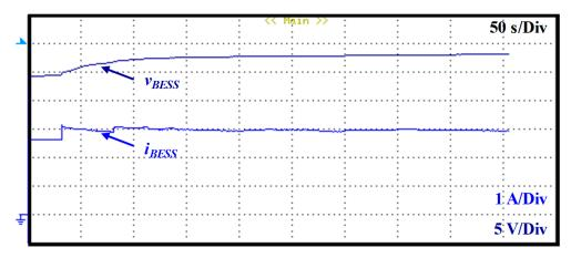
**Figure 18.** Experimental results of the developed multifunctional isolated microinverter: Voltage  $(v_{BESS})$  and current  $(i_{BESS})$  of the BESS during the charging process.
