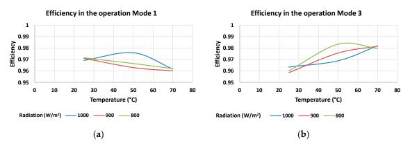
**Figure 11.** Multifunctional microinverter efficiency during: (**a**) Operation mode 1; (**b**) Operation mode 3.
