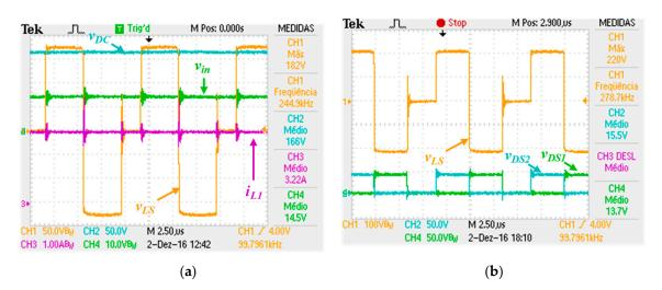
**Figure 16.** Experimental results of the DC–DC power converter: (**a**)  $v_{DC}$ ,  $v_{in}$ ,  $v_{LS}$  and inductor current ( $i_{L1}$ ) with the MPPT algorithm enabled; (**b**)  $v_{LS}$  and the drain-source voltage ( $v_{DS1}$  and  $v_{DS2}$ ) in each MOSFET with the MPPT algorithm enabled.
