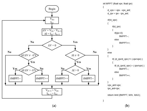
**Figure 4.** Incremental conductance maximum power point tracker (MPPT) control algorithm: (a) Flowchart of the control algorithm; (b) Example of the control algorithm implemented in C language.
