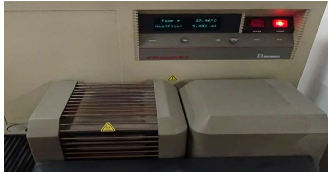
Figure 3.20. DSC-TGA device unit.
