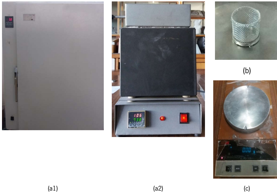
Figure 3.25. (a) The small scale reactor, (b) Cup, and (c) Scale.
