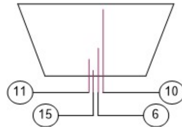
Figure 3.12. Type K thermocouple installed in the fuel bed.
