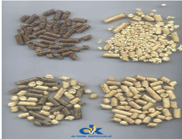
Figure 2.2. Four different qualities of wood pellets (Hansen et al. , 2009).
