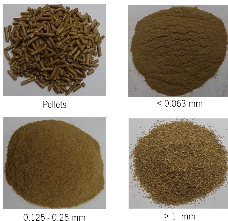
Figure 3.24. Pellets and pine wood particles.
