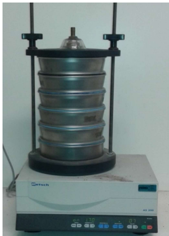
Figure 3.23. Calibrated sieving machine and vibration unit.
