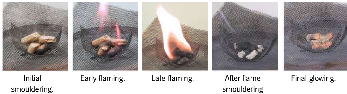
Figure 2.3. Five sequential combustion stages (Olsson, 2006a).
