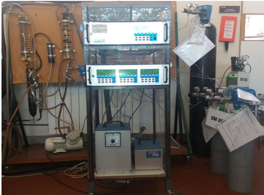
Figure 3.16. Gas emissions collection unit.
