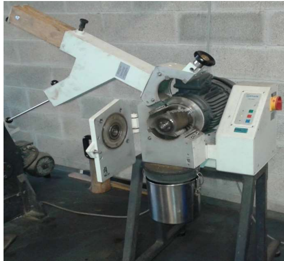
Figure 3.22. Knife mill device.
