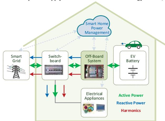
**Fig. 4.** Off-board EV BCS integrated into a smart home, with a parked EV, encompassing the G2V and V2G modes, as well as the possibility of compensating power quality problems related with harmonic currents and low power factor (producing reactive power for the smart home or for the smart grid).
