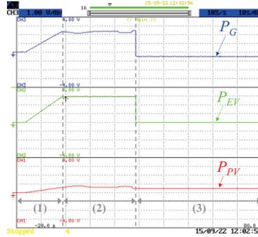
**Fig. 13.** Experimental results when the EV batteries are charged with energy from the power grid and from the PV panels: Power in the grid ( $P_G$ : 1 kW/div); Power in the EV ( $P_{EV}$ : 1 kW/div); Power in the PV panels ( $P_{PV}$ : 1 kW/div).
