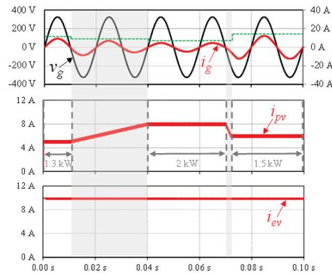
**Fig. 11.** Simulation results when the EV batteries are charged with energy from the power grid and from the PV panels: Power grid voltage ( $v_g$ ); Grid current ( $i_g$ ); Current in the PV panels ( $i_{pv}$ ); Current in the EV batteries ( $i_{ev}$ ).
