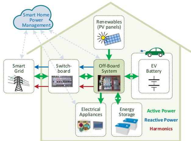
**Fig. 7.** Off-board EV BCS integrated into a dc smart home, with the EV parked and interfacing a RES (solar photovoltaic panels), an ESS (batteries), and electrical appliances through a shared dc-link. The G2V and V2G operation modes are contemplated, as well as the possibility of compensating power quality problems related with harmonic currents and low power factor (producing reactive power for the smart grid).
