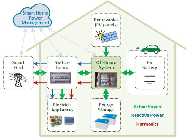
**Fig. 6.** Off-board EV BCS integrated into a hybrid ac and dc smart home, with a parked EV and interfacing a RES (solar photovoltaic panels) and an ESS (batteries) through a shared dc-link. The electrical appliances are directly connected to the ac grid. The G2V/V2G modes are contemplated, as well as the possibility of compensating power quality problems related with harmonic currents and low power factor (producing reactive power for the smart home or for the smart grid).
