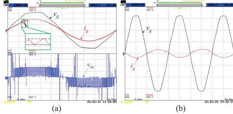
**Fig. 12.** Experimental results when the EV batteries are charged (a) or discharged (b): Power grid voltage ( $v_g$ : 100 V/div); Grid current ( $i_g$ : 10 A/div); Voltage produced by the ac-dc converter ( $v_{ac}$ : 200 V/div).
