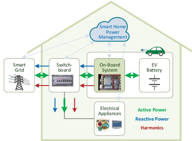
**Fig. 2.** On-board EV BCS integrated into a smart home, encompassing the G2V and V2G modes, as well as the possibility of compensating power quality problems related with harmonic currents and low power factor (producing reactive power for the smart home or for the smart grid).
