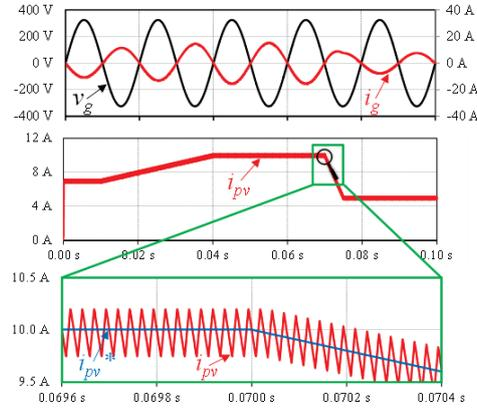
**Fig. 10.** Simulation results when the power grid receives energy from the PV panels: Power grid voltage ( $v_g$ ); Grid current ( $i_g$ ); Current in the PV panels ( $i_{pv}$ ); Reference current for the PV panels ( $i_{pv}^*$ ).
