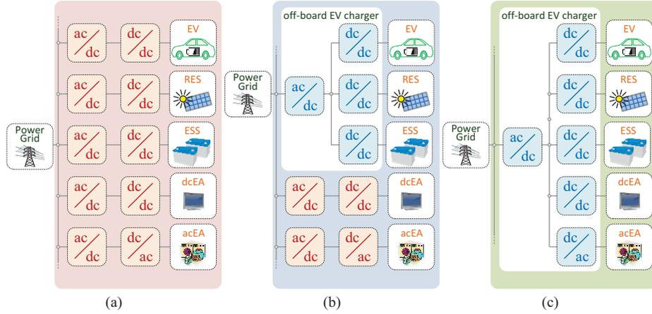
**Fig. 8.** Considered cases: (a) A conventional ac smart home with independent power converters for each technology; (b) A hybrid ac and dc smart home with an integrated EV off-board battery charging system for interfacing a RES and for an ESS, sharing a common dc-link; (c) A dc smart home with an integrated off-board EV BCS, based on a single interface with the grid and with dc-dc or dc-ac converters for interfacing each technology.
