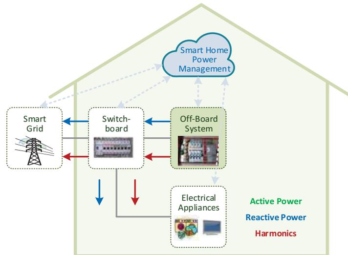
**Fig. 5.** Off-board EV BCS integrated into a smart home, without a parked EV, but with the possibility of compensating power quality problems related with harmonic currents and low power factor (producing reactive power for the smart home or for the smart grid).
