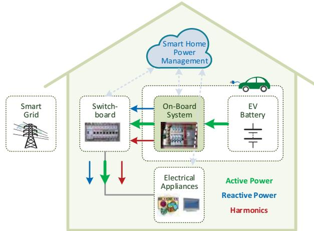
**Fig. 3.** On-board EV BCS integrated into a smart home, encompassing the G2V and V2G modes, as well as the possibility of compensating power quality problems related to power outages (where the EV is used as power supply with the EV batteries as energy source).
