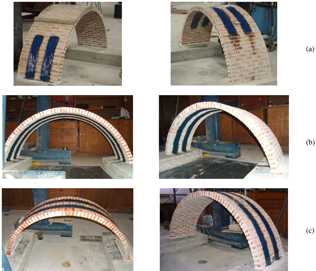
Figure 4. Strengthening arrangements adopted: (a) localized strengthening; (b) continuous intrados strengthening; (c) continuous extrados strengthening.
