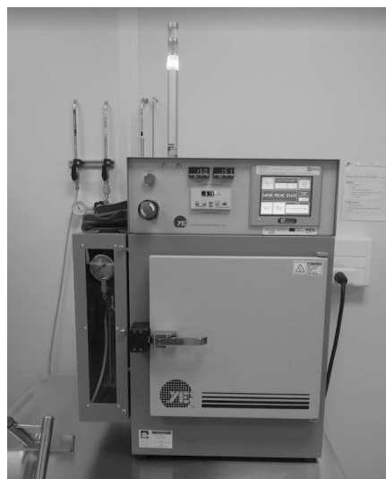
Figure A.7. Vapour prime system.
