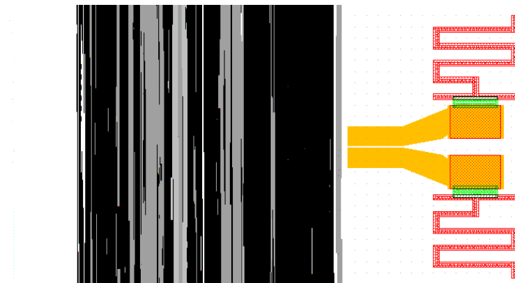
Figure 4.19. Transferred antenna pattern to a CAD design, along with the transmission line.
