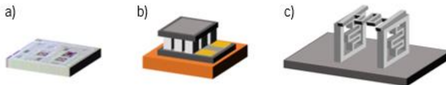
Figure 3.2 a) ASIC designed in house to control the microsystem; b) Peltier device integrated with a heat sink layer of Cu; c) 3D antenna required for this device.
