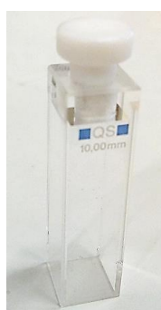
Figure 7.7. High precision quartz glass cell (10×10 mm). Dimensions: 45 × 12,5 × 12,5; volume: 3,5 ml (Hellma Analytics, Germany).
