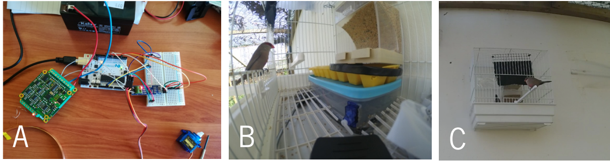
Figure 3. Recapture trap system. (A) Electronic system. (B) Inside view of the birdcage used for the recaptures. (C) Outside view of the birdcage used for the recaptures.
