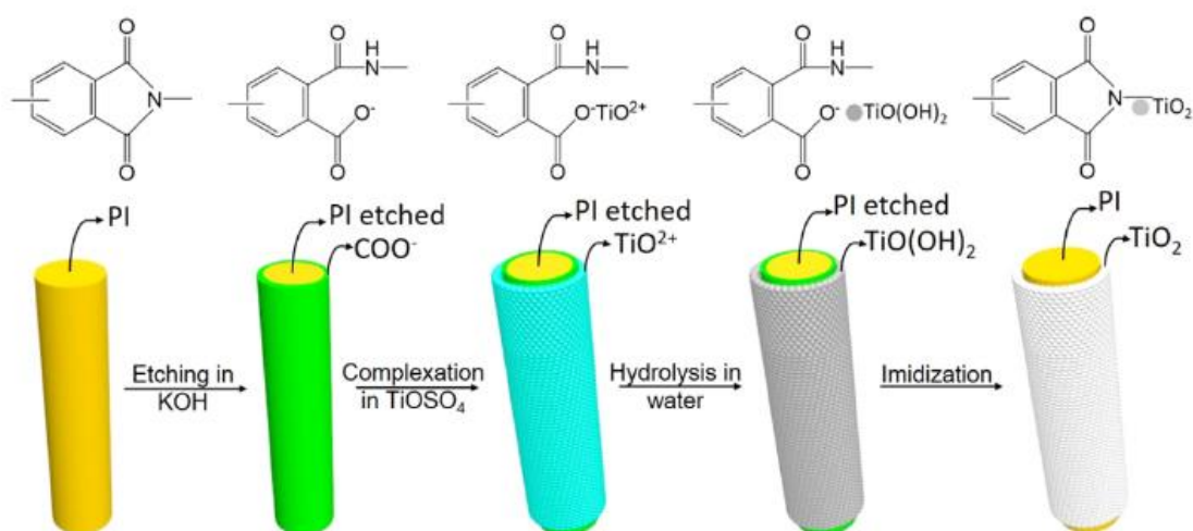
Figure 4 - TiO 2 coating process by alkaline etching and complexation hydrolysis [130].
