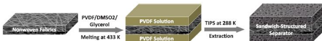
Figure 5 - Schematic representation of a sandwich structure composite separator [131].
