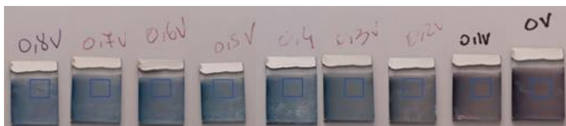
Figure III.3 - Performance of electrochromic material in electrochemical system with 3-electrodes and under the indicated working potential (against Ag/AgCl reference electrode).
