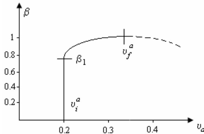
Figure 6 Poisson behaviour proposed by OTTOSEN [6]
