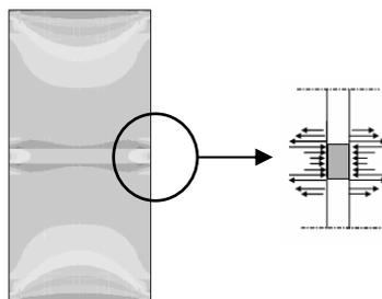
Figure 1 Horizontal stress level developed in block/mortar assemblies
