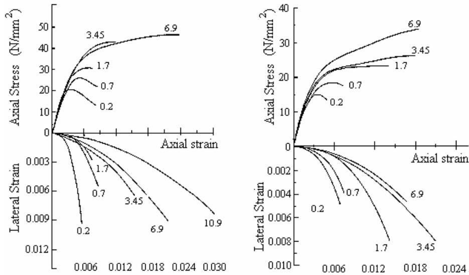
Figure 3 Axial stress and lateral strain diagram for 1:½:4.5 and 1:1:6 mortars
