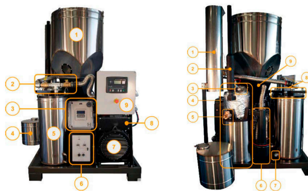
Figure 1. Pilot-scale downdraft reactor. Left: (1) Hopper, (2) Valves to flare and engine, (3) Control unit, (4) Ash vessel, (5) Gas filter, (6) Operational panel, (7) Generator, (8) Wiring box, (9) Grid-tie. Right: (1) Flare, (2) Exhaust stack, (3) Reactor access port, (4) Gasifier, (5) Air inlet check valve, (6) Cyclone, (7) Filter condensate drain bung, (8) Filter lid-locking lever, (9) drying bucket.
