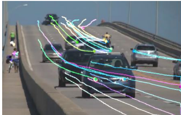
Figure 14.: Lucas-Kanade method using Shi-Tomasi corner detection ( OpenCV Docs )
