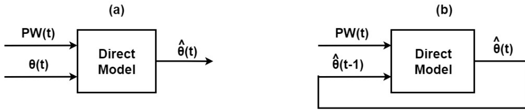
Figure 4.4: Direct model NARX Neural Network diagram for: (a) training and (b) real-time prediction.
