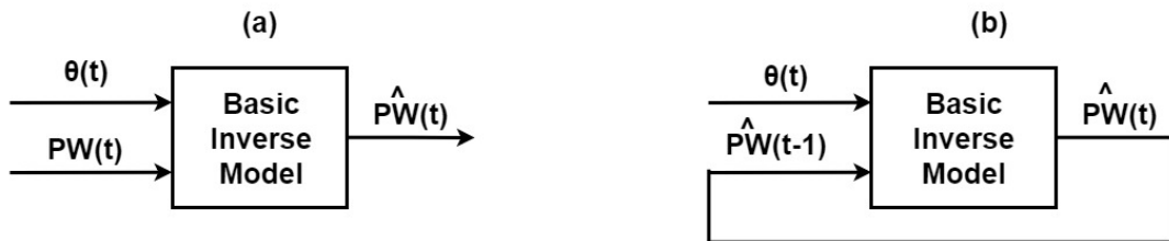
Figure 4.5: Basic inverse model NARX Neural Network diagram for: (a) training and (b) real-time prediction.
