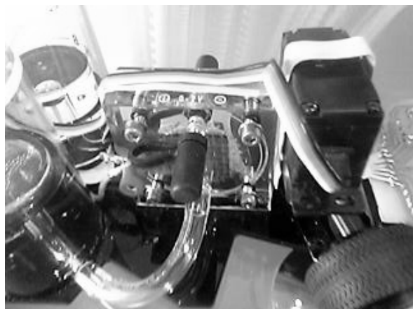
Figure 3. Fuel cell, between the hydrogen and oxygen tanks (on the left) and the servomotor (on the right)
