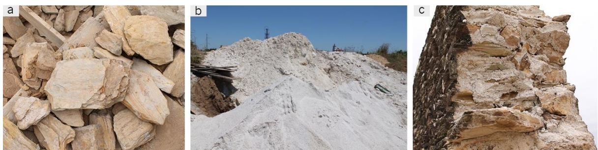
Fig. 9.3 – Images from the case study farm wall building materials: (a) well-defined foliation XO schist stones; (b) clayey soil gathered from the farm; (c) mix of both on the vernacular farm wall cross-section.
