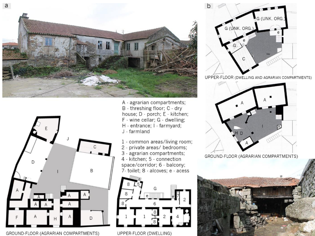
Fig. 5.8 – Examples of farmhouses: (a) lowland large farmhouse with a complex dwelling (Fonte Boa, Esposende) (drawing and image from the author); (b) highland farmhouse with a full organized dwelling [139] (image from a similar farmhouse).
