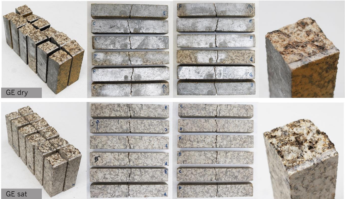
Fig. 7.33 – Images from GE specimens tested for flexural strength (4-points bending test). Rupture plans (right); front and back views (centre); detail from a rupture surface interface (left).
