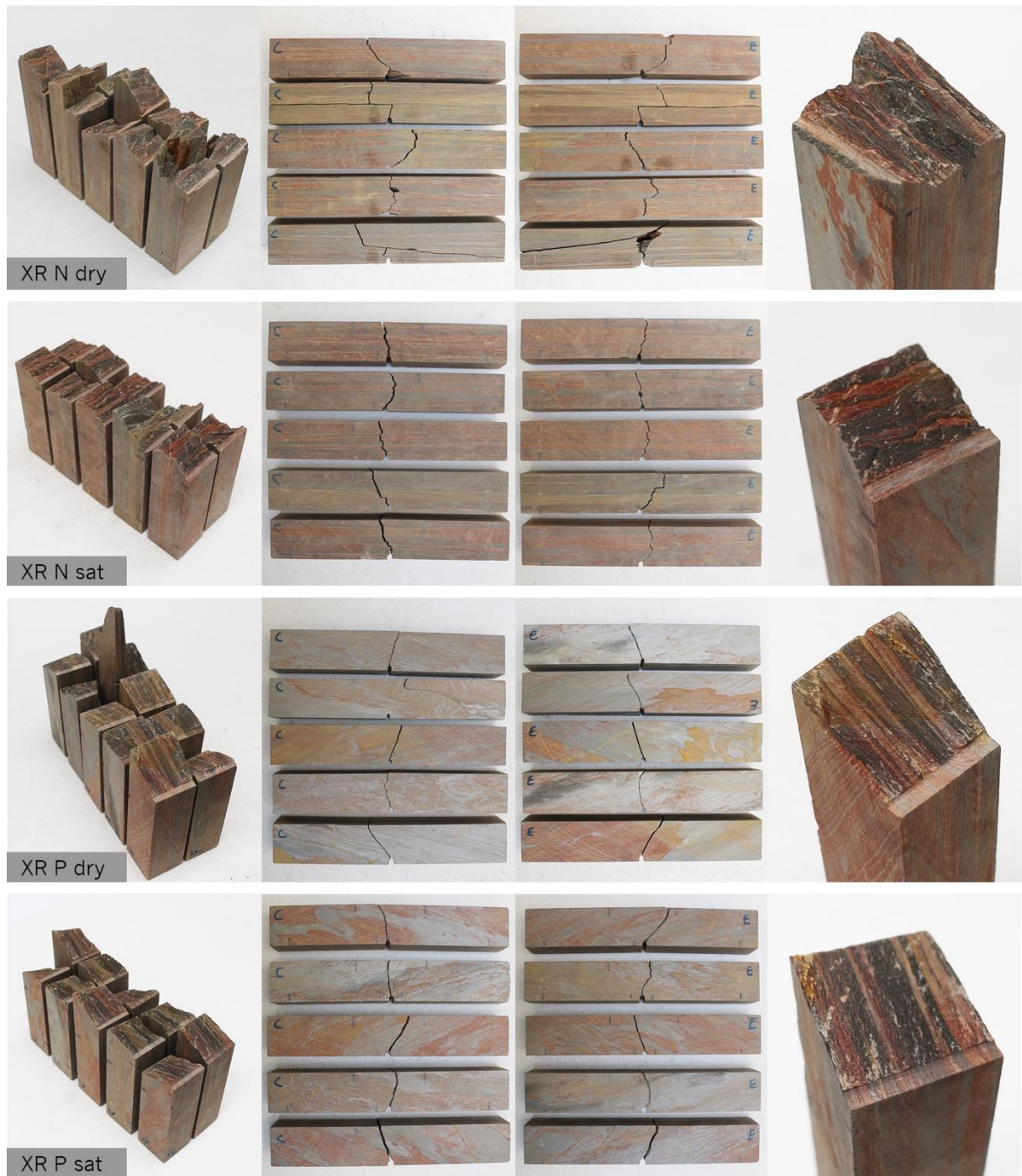
Fig. 7.35 – Images from XR specimens tested for flexural strength (4-points bending test). Rupture plans (right); front and back views (centre); detail from a rupture surface interface (left).
