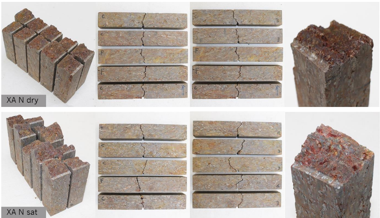
Fig. 7.34 – Images from XA specimens tested for flexural strength (4-points bending test). Rupture plans (right); front and back views (centre); detail from a rupture surface interface (left).
