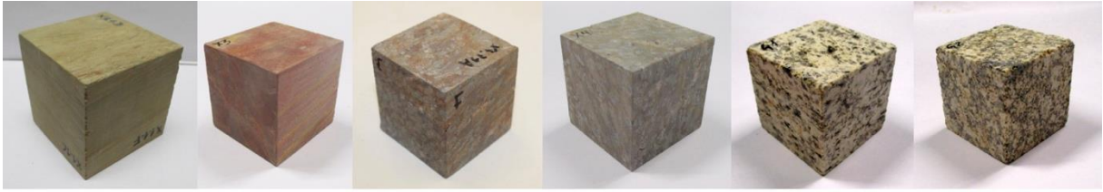
Fig. 7.1 – Examples of 50x50x50 mm 3 specimens of each different type of rock tested (see Section 6.1) for rocks geological characterization.
