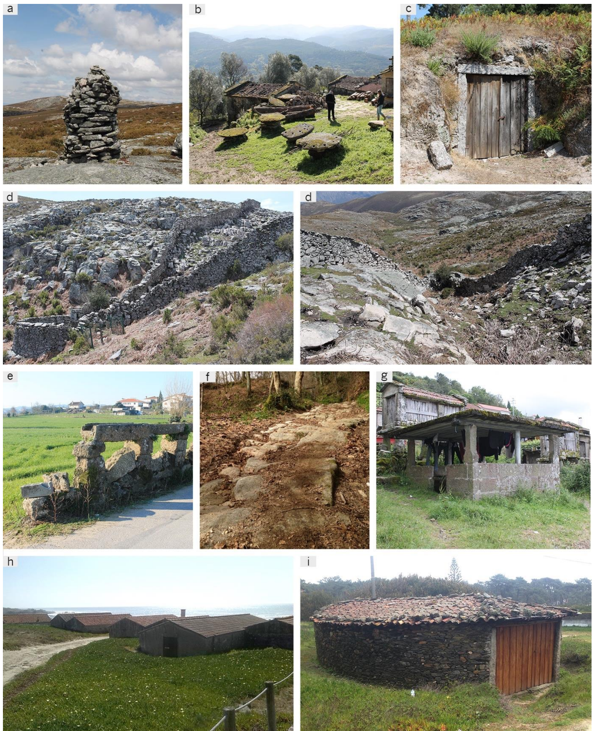
Fig. 5.12 - Examples of production buildings and infrastructures observed during the exploratory visits: (a) landmark (Gavieira, Arcos de Valdevez); (b) common threshing floor with the support for straw granaries named “ canastros ” (Vilarinho do Souto, Arcos de Valdevez); (d) wolf pit trap (Gavieira, Arcos de Valdevez); (e) masonry aqueduct (Barcelos); (f) granite paved rural path (Felgueiras); (g) common washing tank (Padrão, Arcos de Valdevez); (h) fishermen’s sheds (Carreço, Viana do Castelo); (i) “ sargaço ” storage shed (Apúlia, Esposende).
