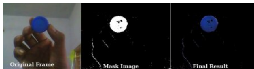
Figure 54: Detection of blue color in an image through the HSV colorspace. Image picked from Python's OpenCV changing color space tutorial .
