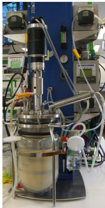
Figure 2. RALF PLUS SOLO bioreactor with bioconversion medium.
