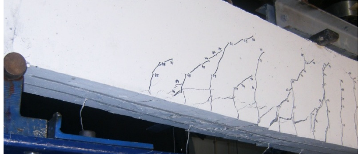
b) Rupture of the CFRP in the beam strengthened with one NSM CFRP laminate (S1L beam)
