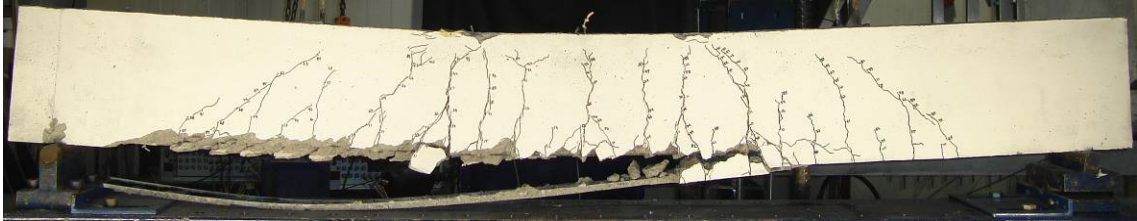
RC beam flexurally strengthened with two CFRP laminates (S2L beam)
