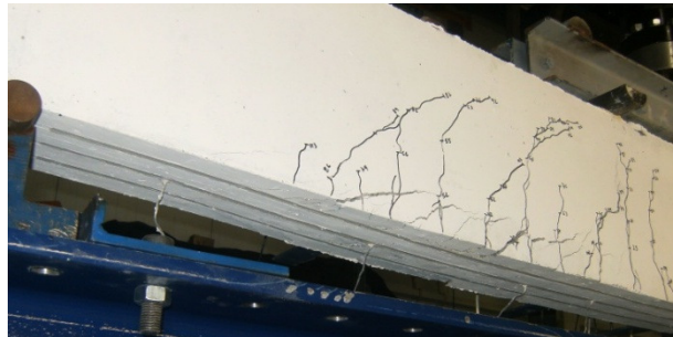
c) Detachment of the CFRP in the beams strengthened with two NSM CFRP laminates (S2L beam)
