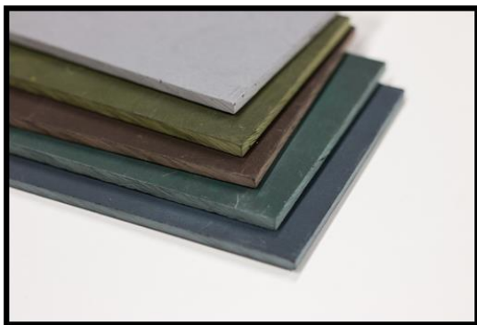
Fig. 5. Composite materials of slate reinforcing bio-epoxy resin
