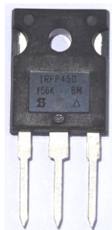
Figura 5.23 - MOSFET IRFP450 da STMicroelectronics [73].
