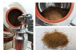
Figure 1. Functionalization of cellulose fibers by spray coating
