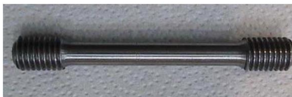
Figure 29 - example of round specimens put in to submitted to monotonic tensile test (Correia, 2014)
