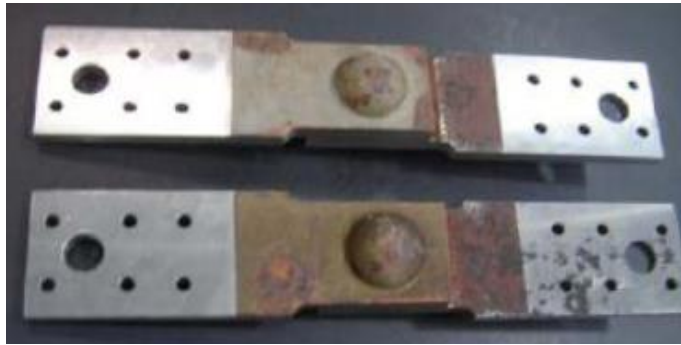
Figure 34 - Photo of the specimens from Trezói bridge (Correia, 2014)
