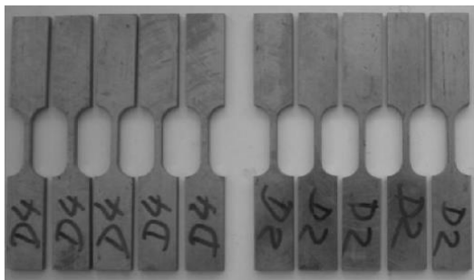
Figure 47 – Example of specimens of material extracted from Fão bridge used (Correia, 2014)
