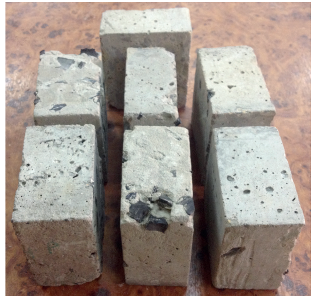
Fig. 5 Specimens of lightweight concretes after 100 freeze-thaw cycles
