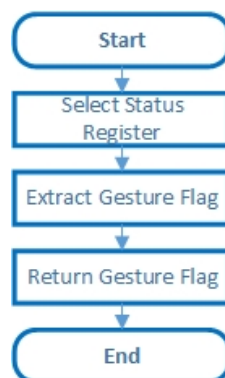
FIGURE 3.12: Gesture detection block.
