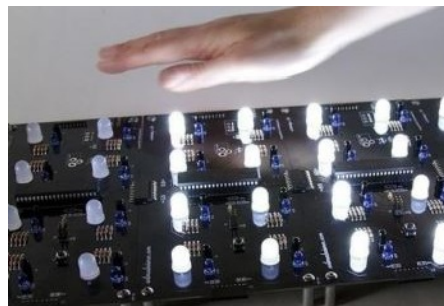
FIGURE 2.38: Contactless Hand Gesture Recognition System [90]
