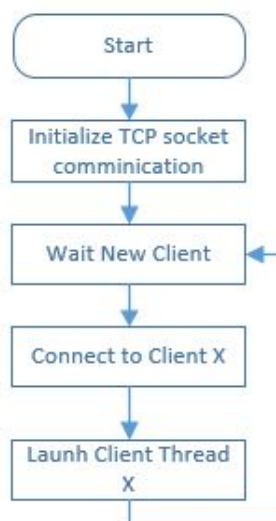
FIGURE 3.24: Main Thread Architecture.
