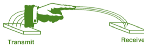
FIGURE 2.13: Transmit Mode Capacitive Sensing [52]
