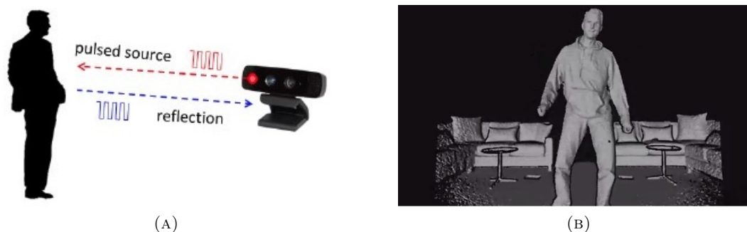
FIGURE 2.21: ToF(Time of Flight) System Schematic (A) [61] and 3D object reconstruction based on a ToF system(B) [62]
